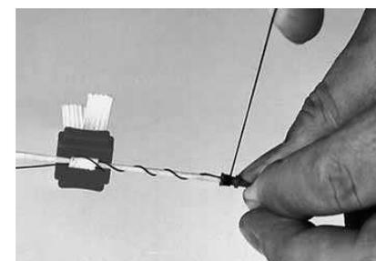
Fix the two halves of the Nocking Point on the string (paying attention to match holes and pins). On each half of the Nocking Point there is a left and a right turning indentation: in this way you will always find one in the correct turning direction. Wrap the yarn around the nocking point, tightly but with not excessive tension.
